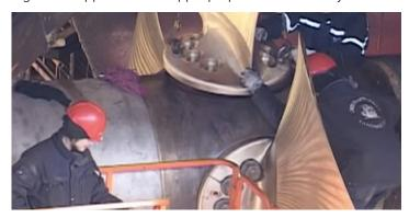
Figure 2b: Rudder bulb and Kappel propeller blades in dry dock
